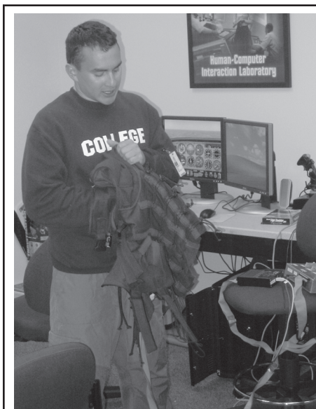
Cadet Hernandez demonstrates his flight vest project. The vest serves as a tactile display to help indicate simple directions, depending on the location of the vibration.
